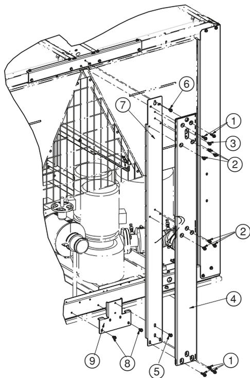
Keep the vertical supports after commissioning the units and re-insert them when the unit is moved.
