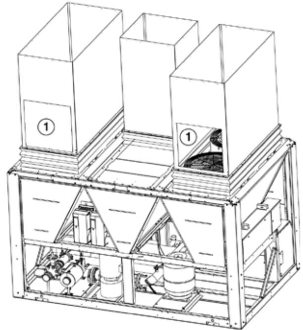
① Fan motor access hatches (provide a 700 x 700 mm hatch) for each single and dual duct
