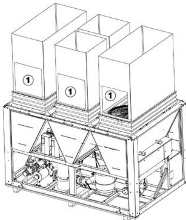
① Fan motor access hatches (provide a 700 x 700 mm hatch) for each single and dual duct
