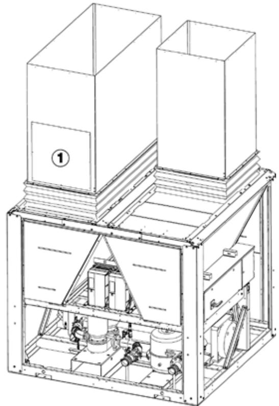
① Fan motor access hatches (provide a 700 x 700 mm hatch) for each single and dual duct
