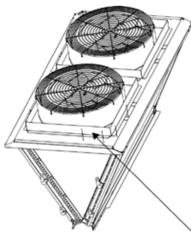
Detail of the duct connection interface frame
