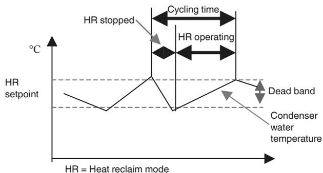
This cycling will lead to a water temperature change in the condenser loop of the heat reclaim condenser. Based on the stability required, the water loop must be more or less significant.
