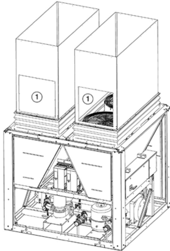
① Fan motor access hatches (provide a 700 x 700 mm hatch) for each single and dual duct
