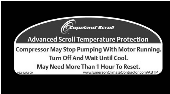
Fig. 20 - Advanced Scroll Temperature Protection Label
