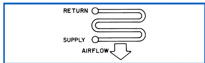
Above is a 4-row coil with a 4-tube face. Note that tubes are staggered in adjacent rows.
