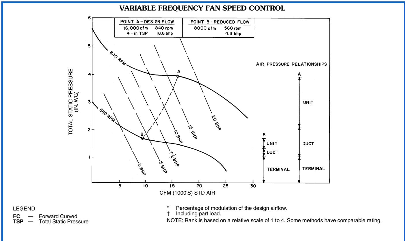
The Variable Frequency Fan Speed Control chart illustrates the results of fan speed reduction as operation shifts from Point A to Point B. If duct pressure begins to fall due to terminal units opening, the duct sensor signals the VFD to increase fan speed.
