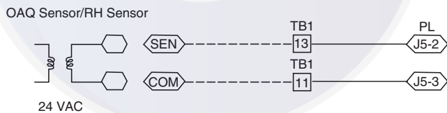
Fig. 62 — Outdoor CO 2 Sensor Connections
