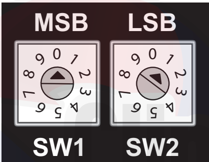
Fig. 82 — RTU Open Controller Address Switches
