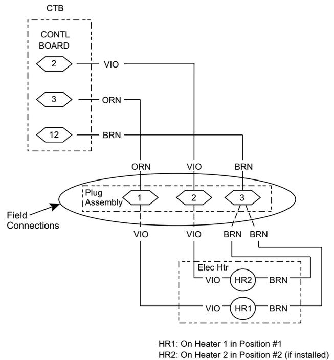
**Fig. 48 — Accessory Electric Heater Control Connections**
