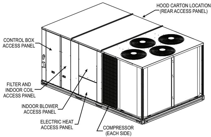
**Fig. 15 — Typical Access Panel and Compressor Locations**
