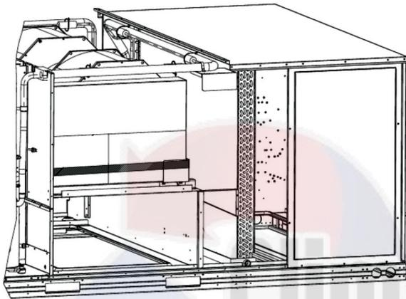
**Fig. 27 — Barometric Hood Box Parts Location**
