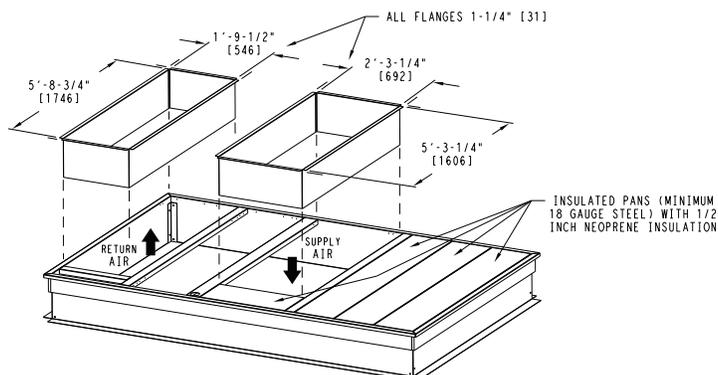
Fig. 16 — Roof Curb Details — 17 and 20 Size Units
