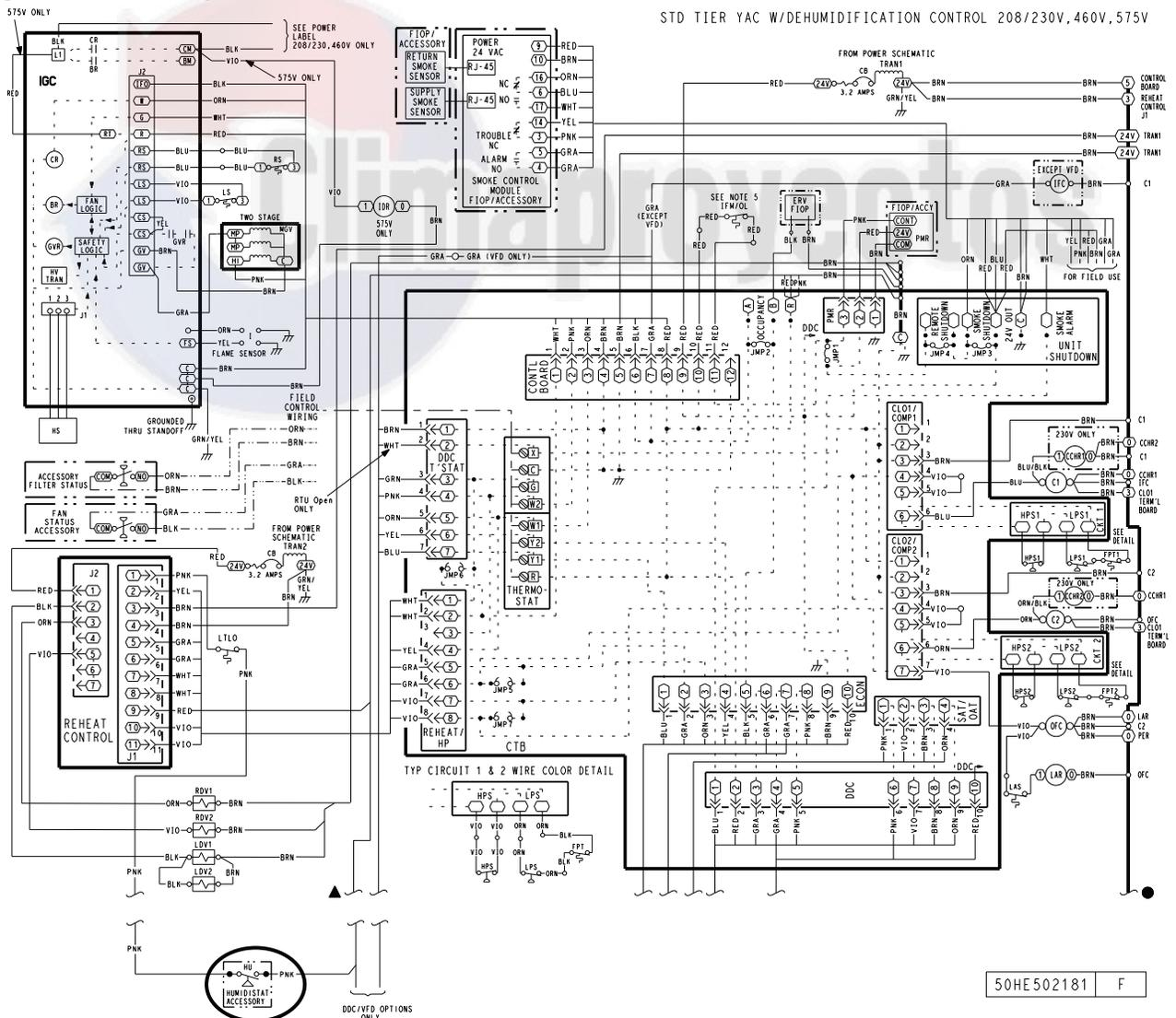
Fig. 51 — Typical Humidi-MiZer<sup>®</sup> Adaptive Dehumidification System Humidistat Wiring
