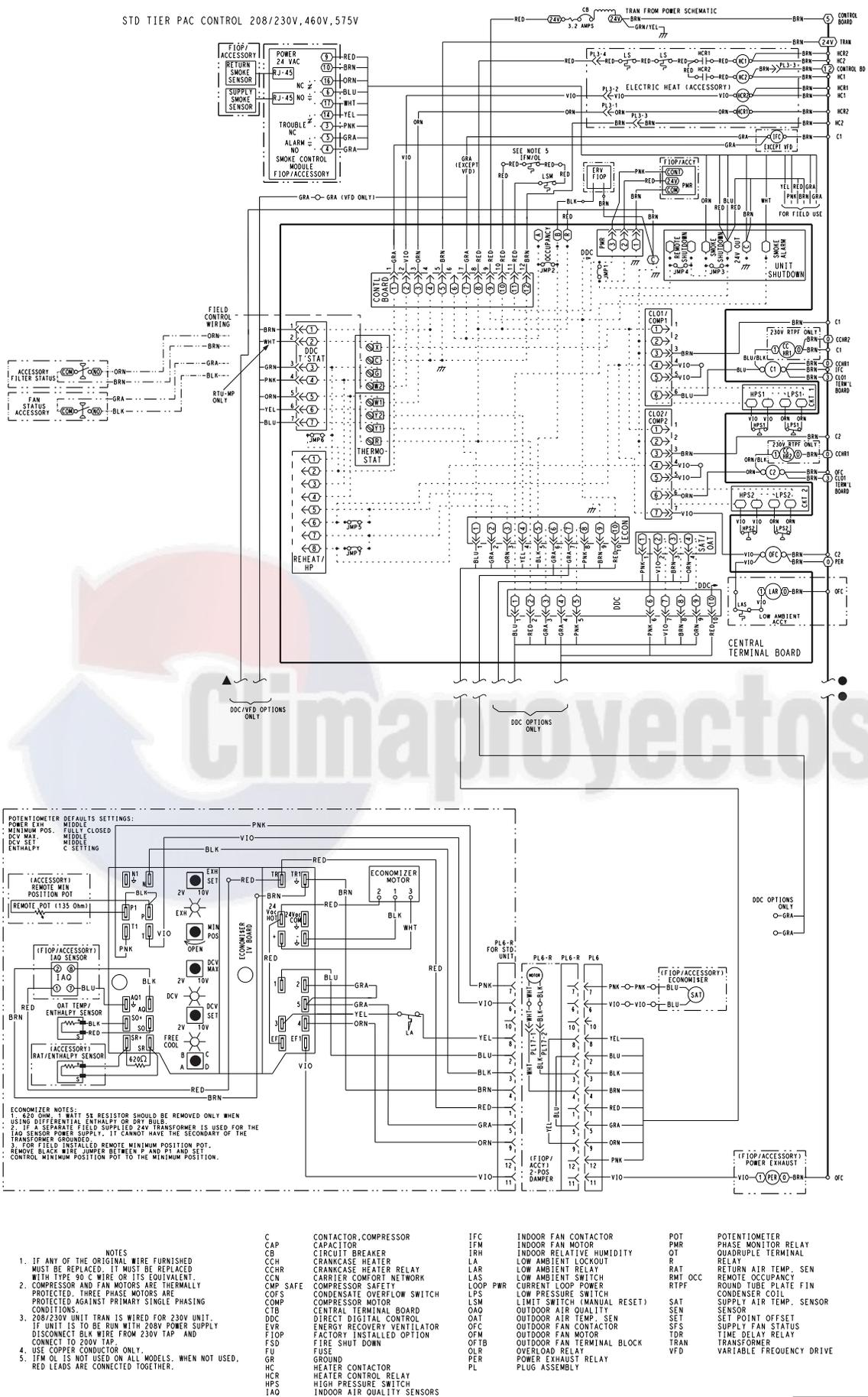
Fig. 63 — 50TC\*\*17-28 Control Wiring Diagram (208/230, 460, 575-3-60)
