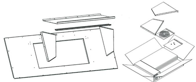
**Fig. 25 — Barometric Hood Parts**
