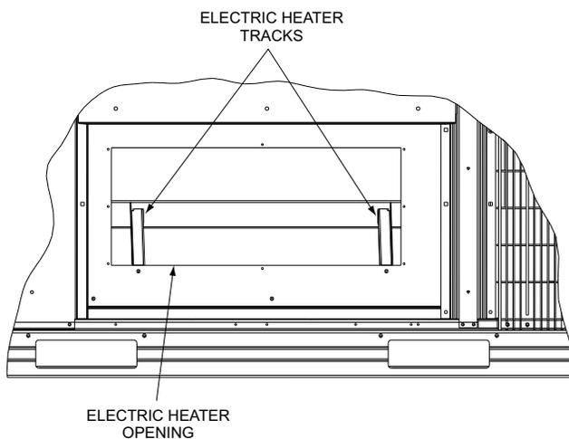
**Fig. 47 — Electric Heater Compartment (Cover Removed)**
