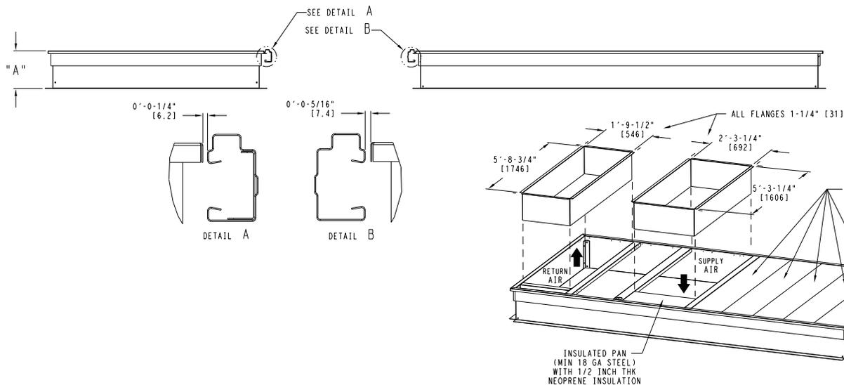
Fig. 18 — Roof Curb Details — 30 Size Units
