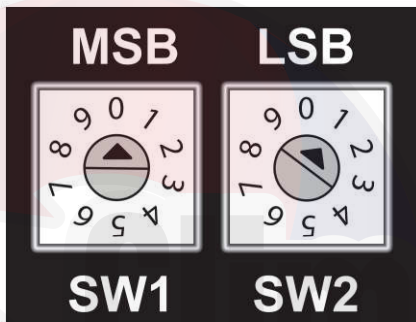
Fig. 86 — RTU Open Controller Address Switches
