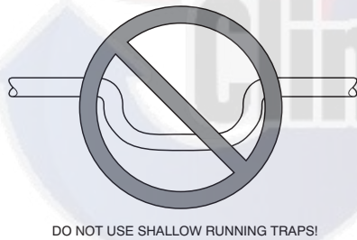
Fig. 18 – Insufficient Condensate Trap
