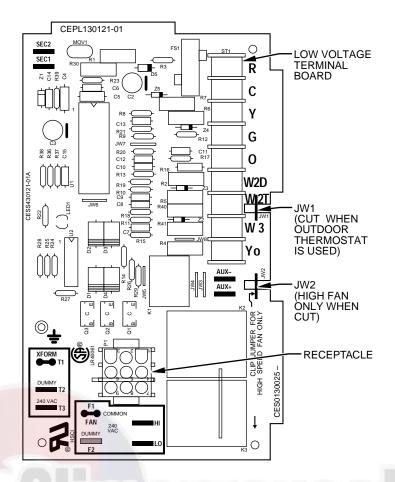
Fig. 27—Smart Heat Printed Circuit Board (PCB)
