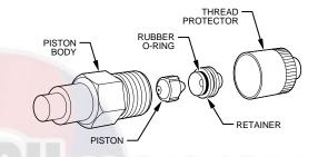
Fig. 24—Refrigerant Flow-Control Device (For FD3A and FG3A)
