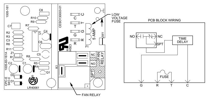
Fig. 29—Fan Coil Printed Circuit Board (CES013C00-00,01 / HK61EA002)
