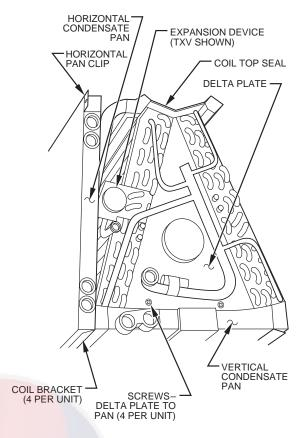
Fig. 43—A-Coil Component Location
