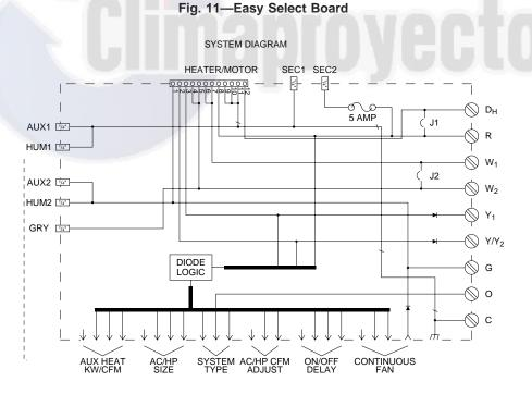
Fig. 12—Easy Select Board Schematic
