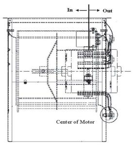
Fig. 41 - Motor Position from Center
