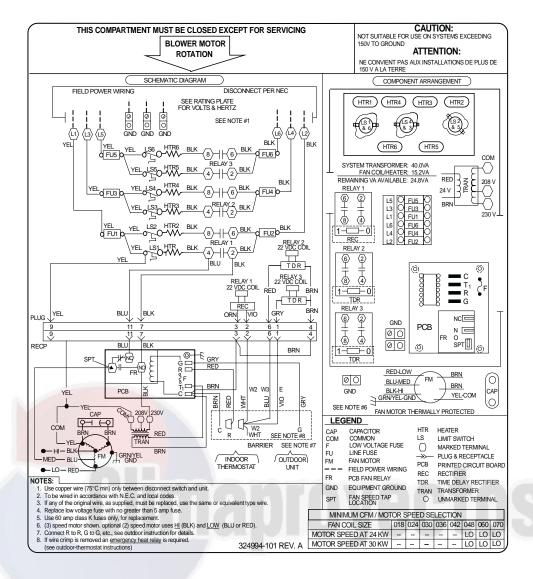
Fig. 31—Wiring Diagram of 6-Element Relay Heater
