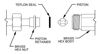
Fig. 42—Refrigerant Flow-Control Device (For FA, FB, and FF) A93530
