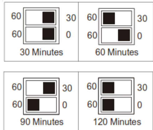
Dipswitch Settings for Selection of Defrost Time
