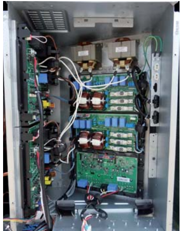
Remove the 3 screws and separate the connector and then separate the double layer structure of Control Box.
