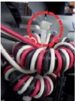
Binds a Comp wire-core to Bracket beam control box using large size Cable-Tie(350mm).
