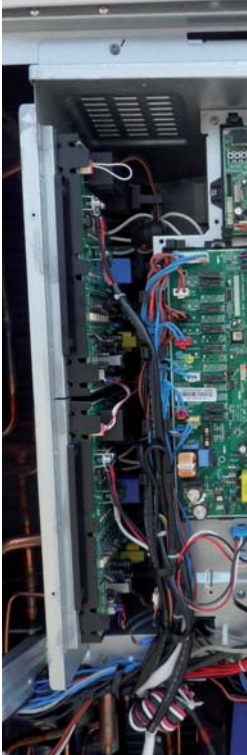
Binds a Comp wire by Holder wire.
