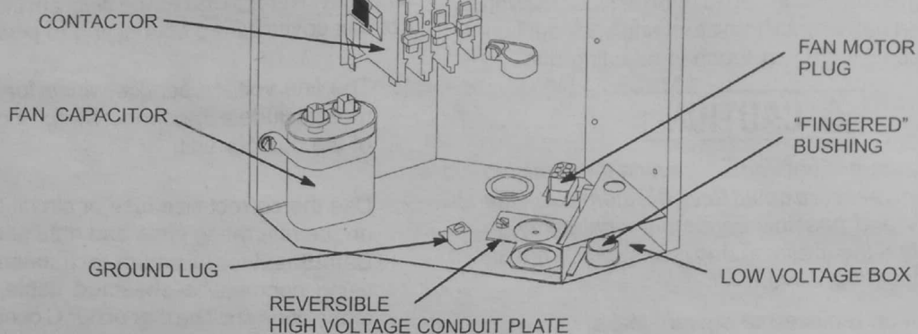
FIGURE 3 - OUTDOOR UNIT CONTROL BOX (036, 048 & 060 MODELS)
