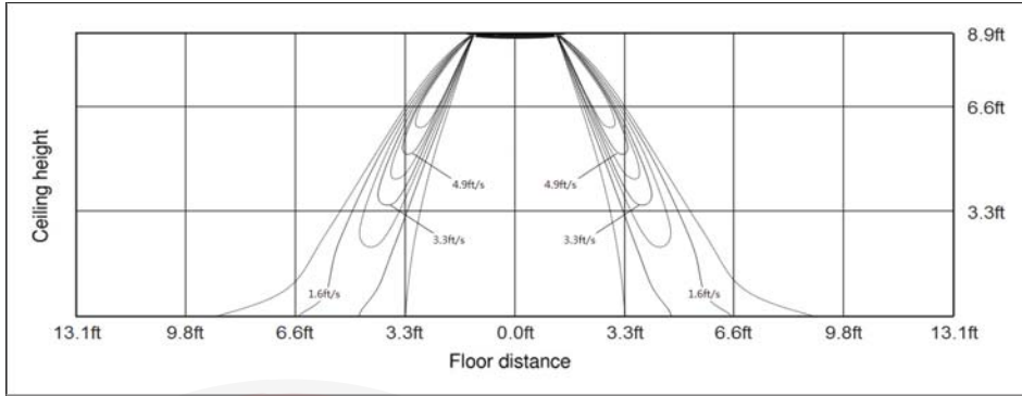
(2) Cooling temperature distribution
