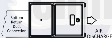
UPFLOW HORIZONTAL RIGHT AIR DISCHARGE
