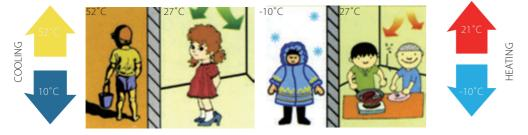
The ambient temperature operating range is 10°C to 52°C in cooling mode and -10°C to 21°C in heating mode.
