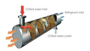
For shell-tube heat exchanger, the module adopts the new helical baffle design to avoid the rectangular place of water dead zone, greatly improve the heat exchange efficiency.
