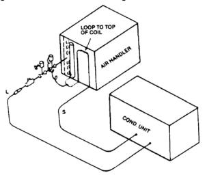
Figure 14: Coil Below Condensing Unit
