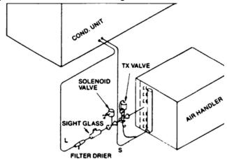
$\ensuremath{\mathsf{NOTE}}$ : PIPING ACCESSORIES SHOWN SHOULD BE MOUNTED AS CLOSE TO AIR HANDLER AS POSSIBLE.
