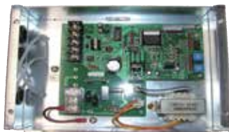
Modbus® Interface TCB-IFMB641TLE
