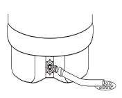
ADANGER: Before manually operating the relief valve, make certain no one will be exposed to the hot water released by the valve. The water drained from the tank may be hot enough to present a scald hazard and should be directed to a suitable drain to prevent injury or damage.
