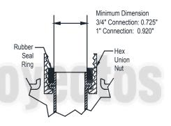
The hot water connection fitting must have a inside diameter greater than the minimum shown in the picture above.
